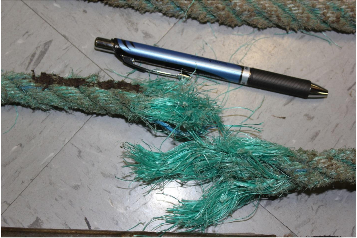
Photo #4 frayed rope
