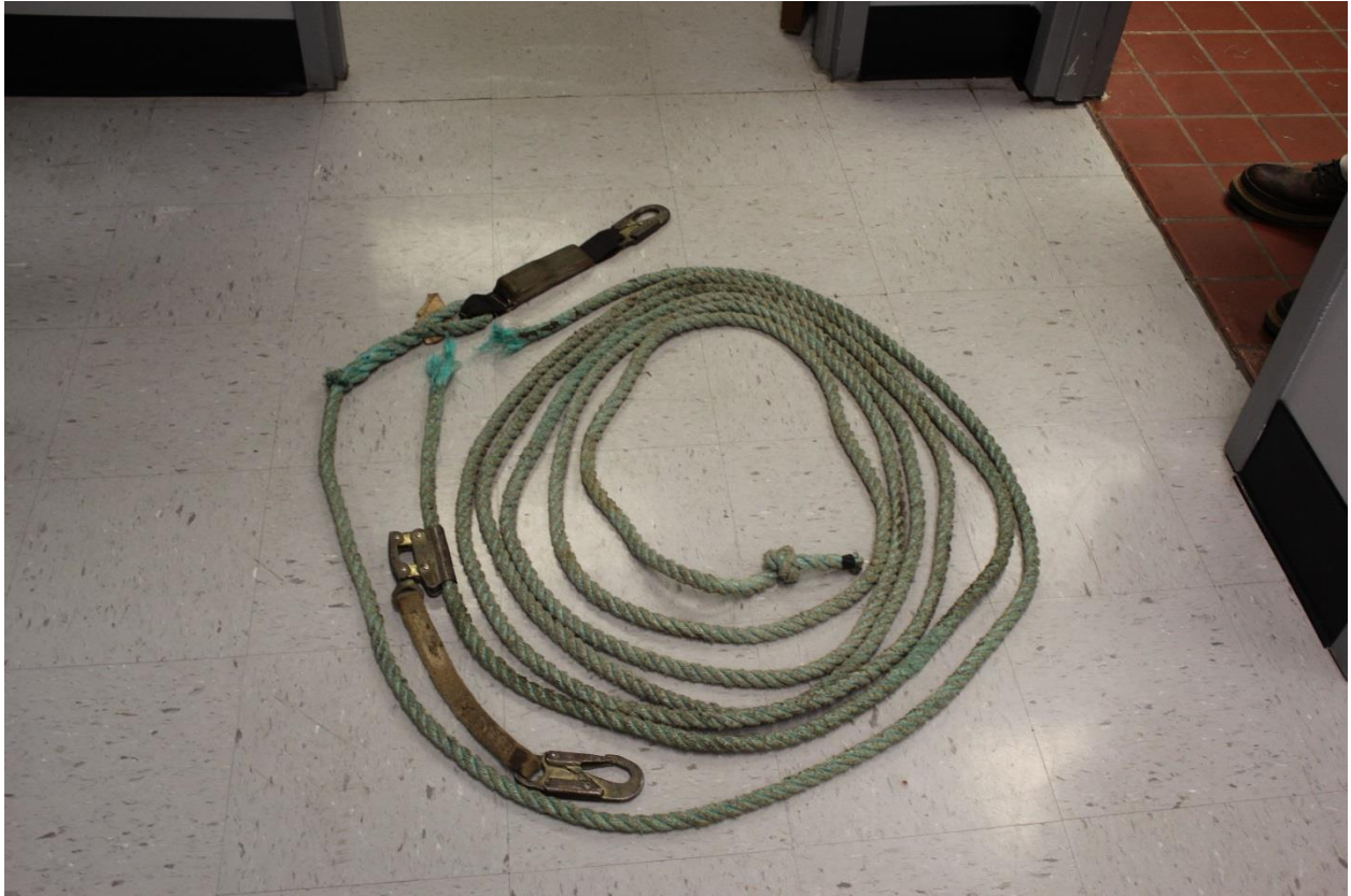
Photo #3 the worn lanyard with rust.
