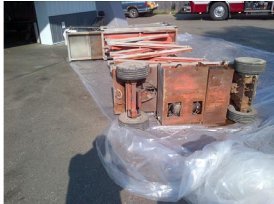
Figure 1. Incident site showing overturned scissor lift
