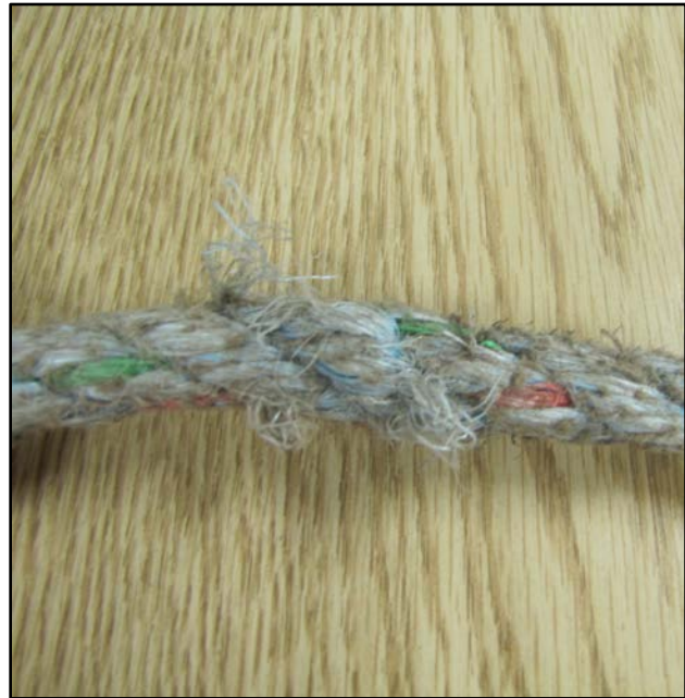
Photo 4. Damaged fibers in laborer's 50-foot lifeline ( Photo courtesy of NCDOL/OSH )
