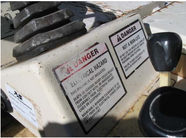
Photo 3 Warning Plate Inside Cab (courtesy of OSHA)
